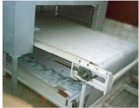
BELT CONVEYOR FOR PAINT BOOTH SYSTEM LENGTH OF CONVEYOR - 20 Mtrs.
